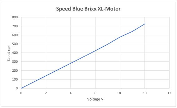
Fig 7: Speed diagram Blue Brixx XL-Motor
