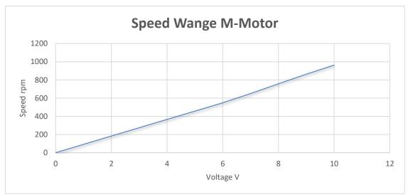
Fig 27: Speed diagram of Wange M-Motor
