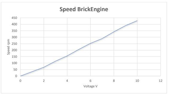
Fig 11: Speed diagram Brickengine V1
