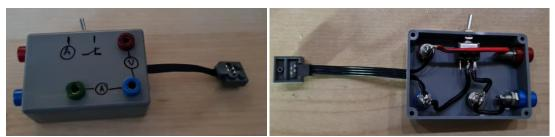
Fig 30: Measuring box for Power Functions motors
