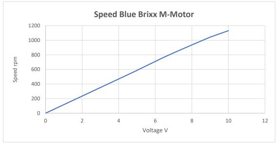
Fig 5: Speed diagram Blue Brixx M-Motor
