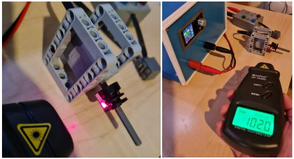
Fig 31: Reflectors on rim and measurement
