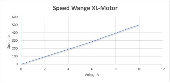
Fig 29: Speed diagram of Wange XL-Motor
