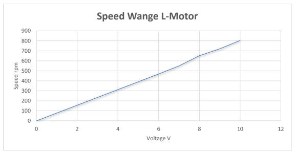
Fig 28: Speed diagram of Wange L-Motor
