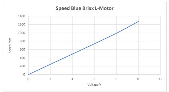
Fig 6: Speed diagram Blue Brixx L-Motor
