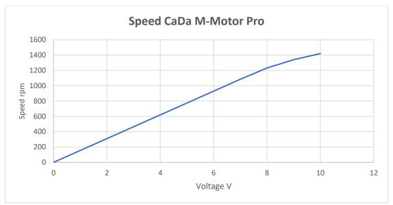
Fig 23: Speed diagram of CADA M-Motor Pro
