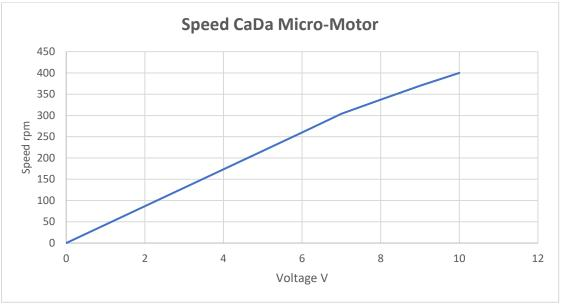
Fig 24: Speed diagram of CADA Micro motor
