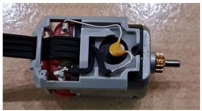
Fig 26: Inner workings of a Wange M motor
