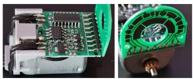
Fig 16: Control electronics (left) and angle encoder (right) of the CaDa servo
