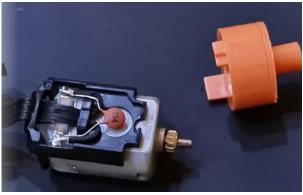
Fig 3: Blue Brixx L-Motor Interior
