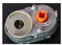
Fig 17: Gear and contact plate of the angle encoder
