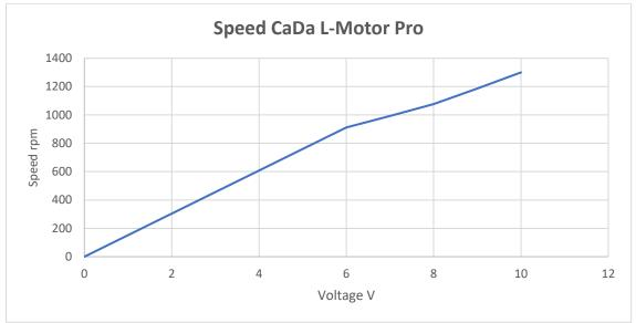
Fig 22: Speed diagram of CADA L-Motor Pro
