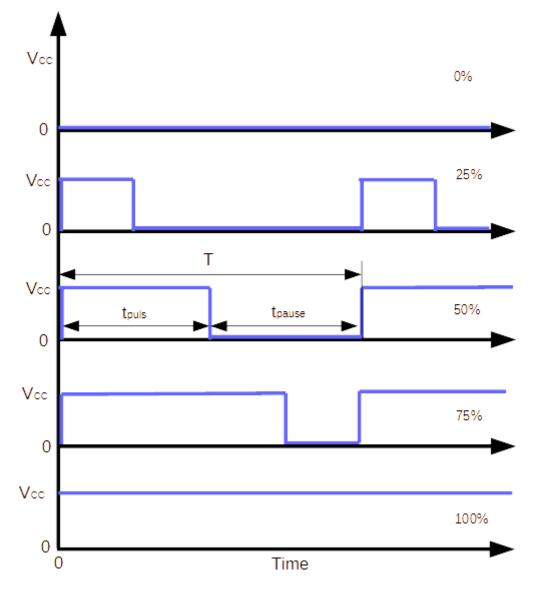
Fig 2: Different duty cycles of a pulse width signal
