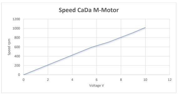
Fig 21: Speed diagram of CADA M-Motor
